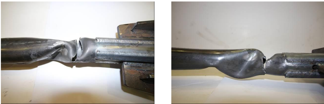
Figure 2.17. Fractured main brace of TinT#2
