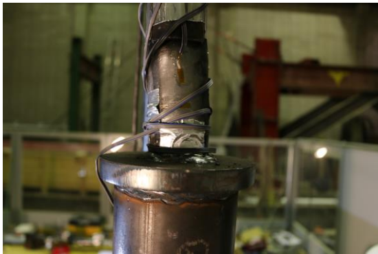
(c) Rotation of the top edge tube (Loading end)
