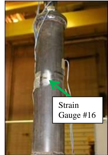
(b) Strain gauge#16 (Center Tube)
