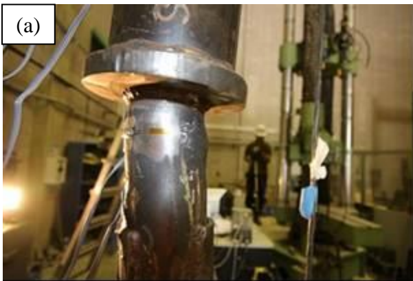
Figure 4.42. Out-of-plane rotation of the lower connector plate and necking of the edge tube to the fixed end at 2.5% SDR.
