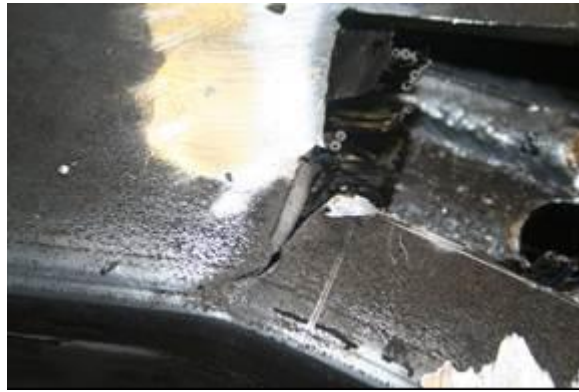
(c) Fractured slotted end of the outer tube
