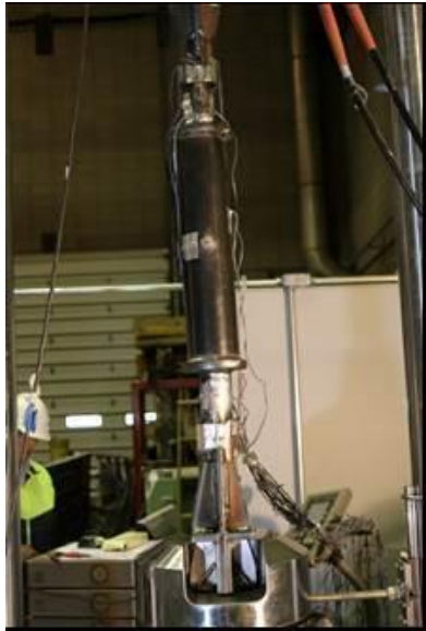
(c) Out-of-plane buckling shape
