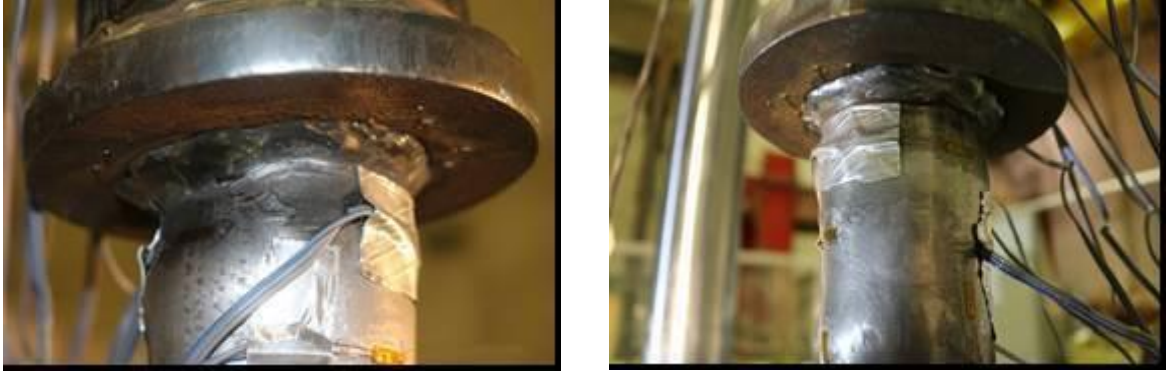
Figure 4.34. Bulging (necking) of the edge tube to the fixed end at 2.00% SDR in compression
