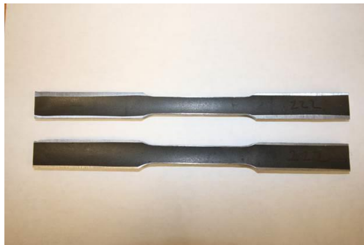
Figure A.3. Coupon specimens prior to the test
