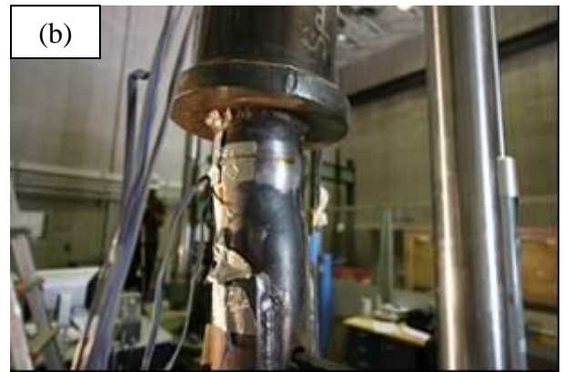
Figure 4.42. Out-of-plane rotation of the lower connector plate and necking of the edge tube to the fixed end at 2.5% SDR.
