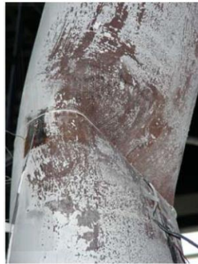
(c) Local buckling of a CHS specimen at plastic hinge location
