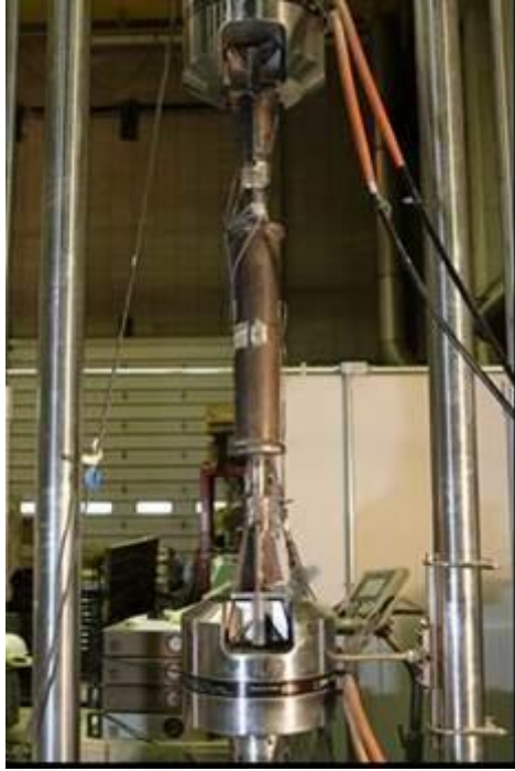
(a) Out-of-Plane Buckling
